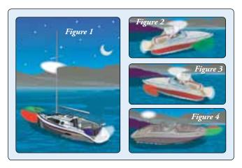
A masthead light and a sternlight visible from a distance of at least two miles away. The masthead light must be higher than the sidelights as shown in *Figures 1, 2, and 3*.
